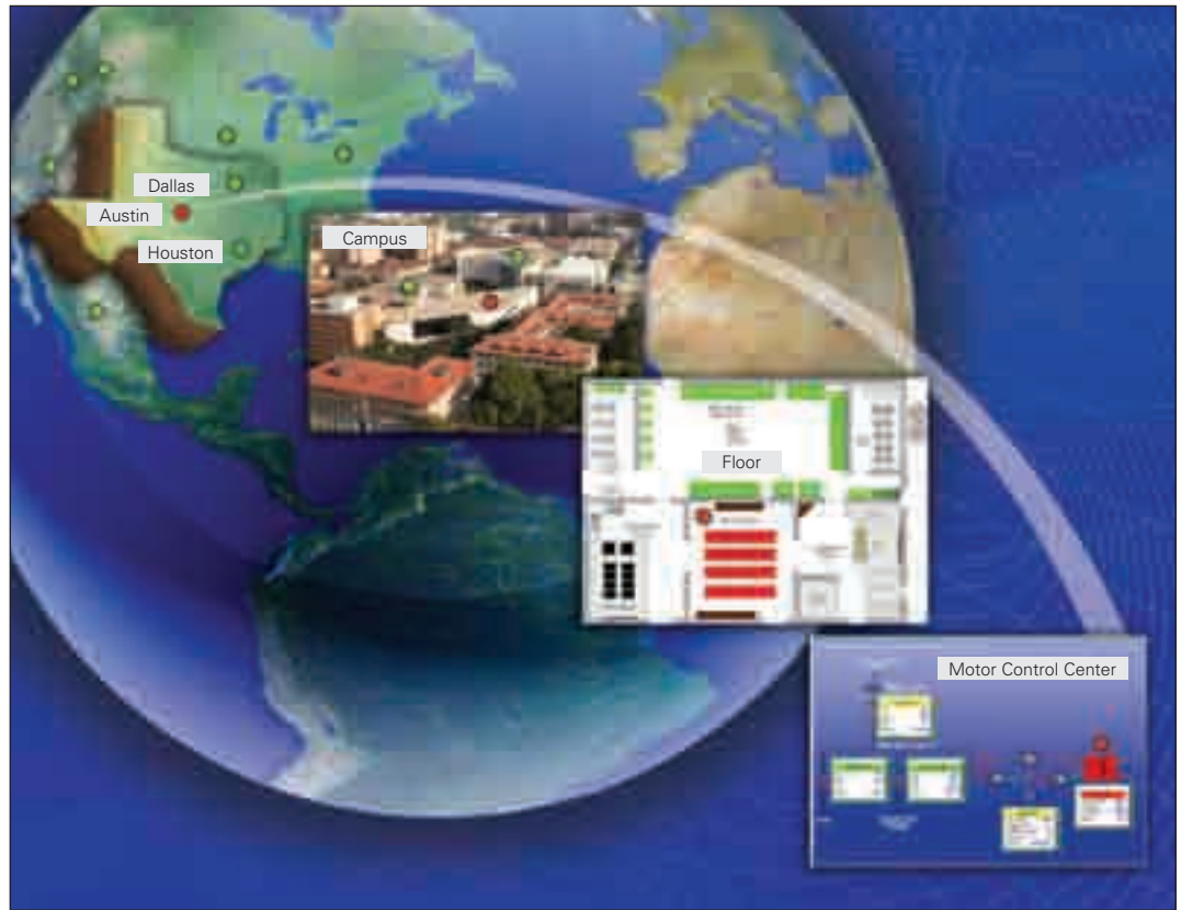
Use Layout Manager to import world and city maps, including their facilities and specific gear that is monitored by the Power Xpert Software. They can design an easy drill-down user interface that also allows an alarm to bubble-up when devices trigger alarming events.
